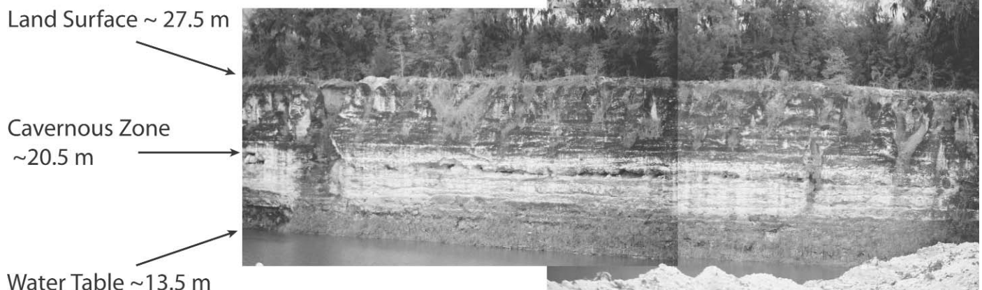
Figure 9. Photo of highwall at Haile Quarry near Gainesville in north-central Florida. The highwall is approximately 14 m tall, and the land surface is approximately 27.5 m above mean sea level. Note the laterally continuous cavernous zone 7 m below the top of the highwall at +20.5 m (Figures 5a and 9 of LaFrenz et al. , 2003).
